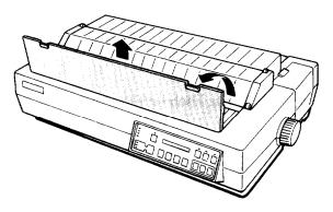
Open the paper guide cover as shown in the illustration. Then raise the rear of the cover slightly and lift the cover away from the printer at a slight upward angle.
